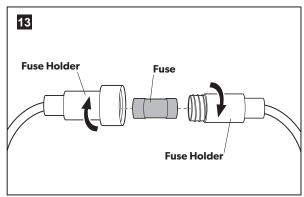
Refrigerators equipped with a vent fan(s) include an inline fuse on the wire supplying power to the fans(s). This wire is connected to the 12 VDC terminal block supplying DC power to the refrigerator controls.
