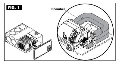
• Inspect the chamber and vent system for holes or excessive corrosion.
